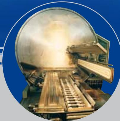
Electric arc evaporators are mainly applied on batch coaters. We have the ability to produce electric arc evaporators of both planar configuration devices with target length up to 1.15 m and tubular form with target length up to 4.0 m (U-shaped) and up to 1.6 m (linear).
