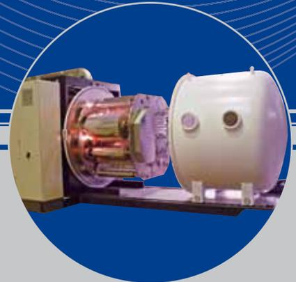
Preliminary drying and degassing of substrate materials in vacuum before deposition will guarantee high quality coating. In particular, this applies to polymer films, synthetic fabrics and non-woven materials. After such treatment the material will not cause any problems during coating. That is why in many cases we recommend that our customers purchase a set of two
