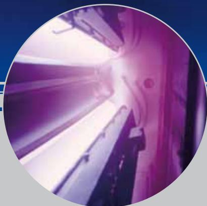
Planar and cylindrical magnetron sputtering devices have been developed and put on sale. Both single and double magnetron configurations can be applied. These can feature clamped or bonded target with direct or indirect cooling, and with external or internal cooling water and power connections. Length of targets is up to 3.0 m.
