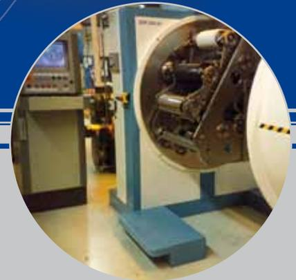
Vacuum laminators play a critical role in the production of flexible printed circuits based on polyimide film. Vacuum laminators have been designed for double-sided lamination of photo resist polymer material onto flexible polyimide printed circuits. Appropriate temperature and pressure
