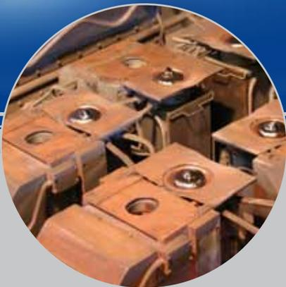
Evaporation boats for the deposition of copper, silver and gold at high rates can be demonstrated as our major achievement in the area of thermal evaporation.
