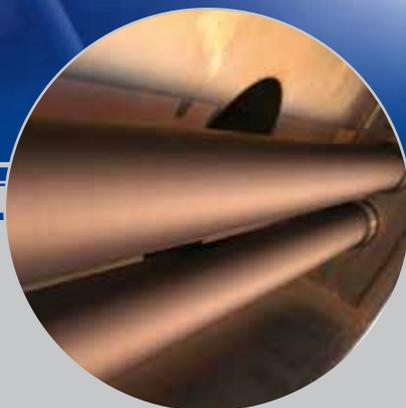
We have developed several types of cylindrical rotary magnetrons, particularly: with rotary targets or rotary magnetic fields.
